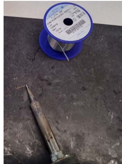
Solder both ends for each wire (2-3 mm long).
